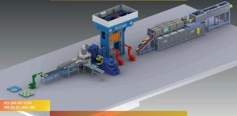
Completely automatic lines: Furnaces; Induction heaters; Presses; Manipulators; Robots; Ring rolling mills
